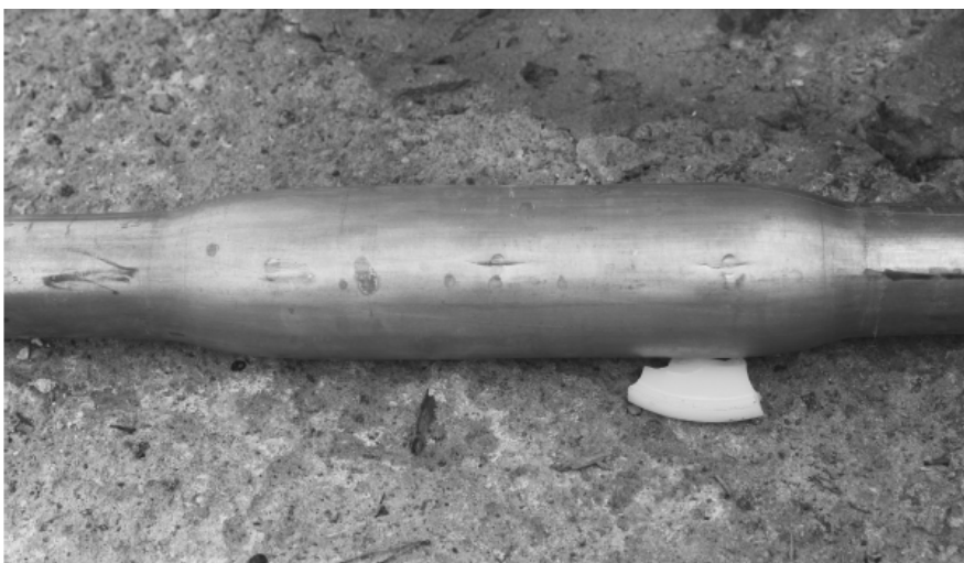
Fig. 8. Liner expanded through the failure of retarded HMX charge initiation from the axial detonator
